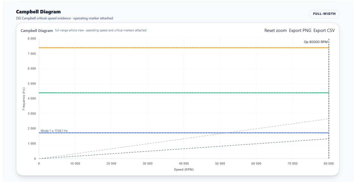
Figure 2. AURA Campbell-diagram screen with the operating-speed marker and modal evidence exposed. Dynamic-screening example supplied by Breshev Engineering.
